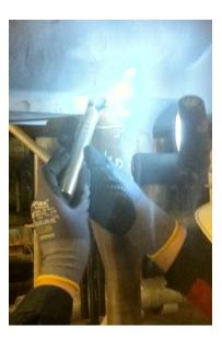
Prerequisite for a steady hardness test: Surface must be clean and smooth according to spec. (DIN 50159-1). In addition the procedures described in the standards need to be considered (DIN 50159, ASTM A 1038).
