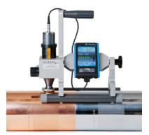
There are not many alternatives at hand compared to the UCI-Method to be used at the same time on soft Aluminum (here EN573) as on hard metal with test loads between 1N and 8.6N (motor probes) and 10N to 100N (handheld probes).
