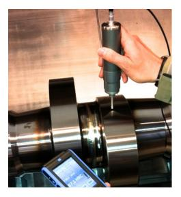
**SONO-8M, HV0.9 (8.6N):** general production control in metal fabrication industries, testing of gear teeth in heat treatment shops (induction hardening)
