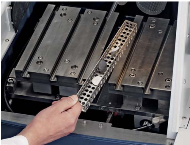
Parts tray catches small samples for easy retrieval.
