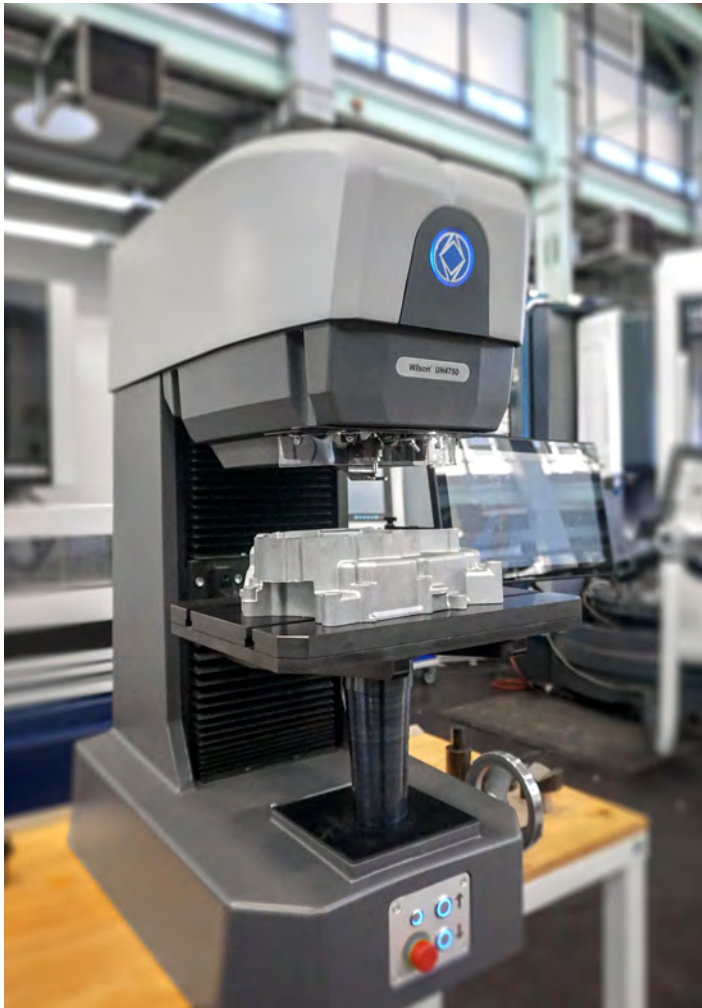
Wilson UH4750 with AlMgSi casting
