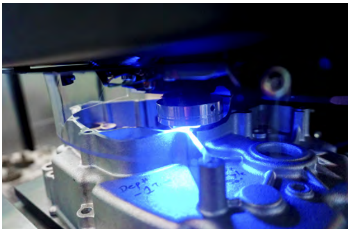
Wilson UH4750 with AlMgSi casting
