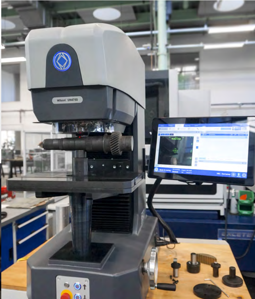
The UH4000 comes with an anvil extension to enable testing of smaller or cylindrical parts.
