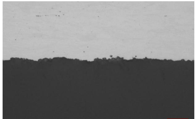
Inside diameter of a steel washer mounted with EpoKwick FC showing no shrinkage gap.
