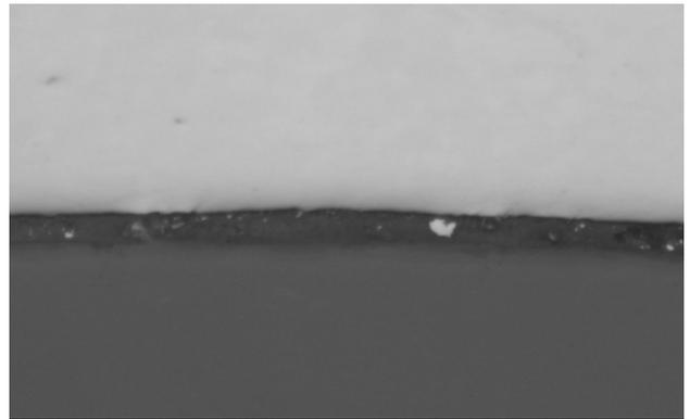
Inside diameter of a steel washer mounted with Nearest Competitor epoxy produces shrinkage gaps.
