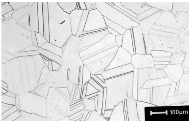
Figure 5: EBSD pattern and microstructure of cartridge brass: top: EBSD pattern for Cu - 30% Zn - PQL: 221 \pm 8.6 ; bottom: microstructure of wrought, annealed Cu - 30% Zn etched with equal parts hydrogen peroxide (3%) and ammonium hydroxide.
