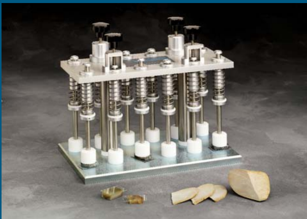
The PetroBond® Thin Section Bonding Fixture is designed to accurately control the thickness of the bonding media between the specimens and glass slides.
