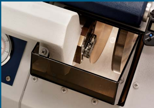
Glass slide mounted specimen is resectioned on the diamond cutting blade. The grinding blade (right) reduces the specimen thickness without removing the specimen after resectioning.
